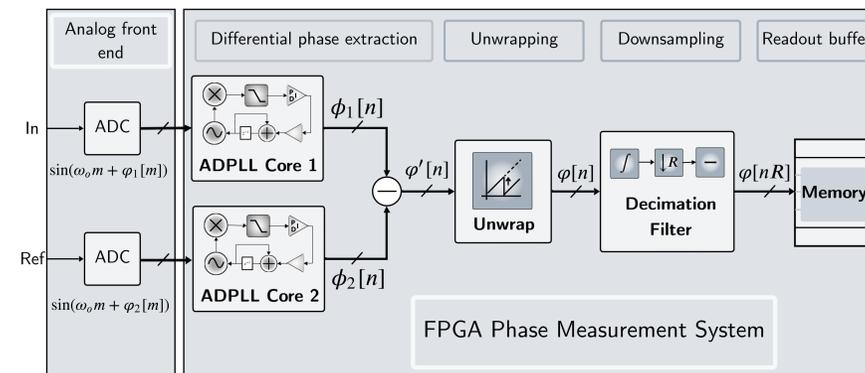
Figure 4. Phase measurement principle: Independent ADPLL cores track input and reference signals. The differential phase measurement  $\Delta\phi = \phi_1 - \phi_2$  provides the phase readout.
