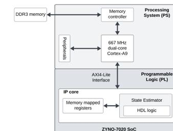
Figure 9. Nav filter operations on FPGA-SoC. Figure 10. FPGA v. double-precision simulations.
