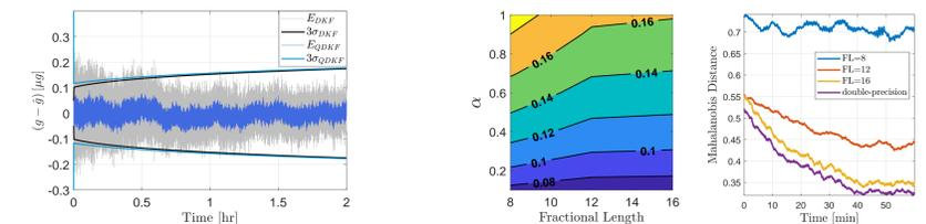
Figure 7. Estimation errors and  $3\sigma$  bounds from DKF and QDKF with 12-bit measurements. Figure 8. Steady-state: (Left)  $1\sigma$  contours. (Right) Mahalanobis distance of estimates.
