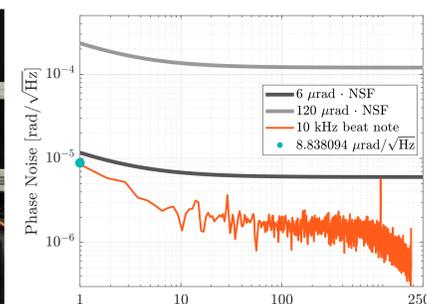
Figure 6. Phase noise performance compared to  $6 \mu\text{rad}/\sqrt{\text{Hz}}$  LISA requirement.
